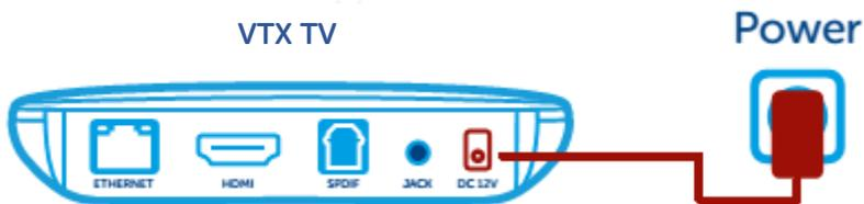
Connect the AC adapter to the VTX TV box, then insert the power plug into your wall socket. The VTX TV box will immediately turn on when power is connected.
