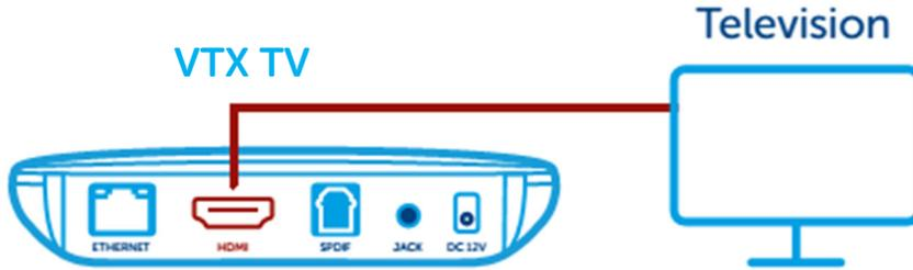
Connect one side of the HDMI cable to your VTX TV box, and the other side to your TV. If your TV has multiple available HDMI inputs, please set your TV accordingly. Note that the HDMI cable carries both audio and video signals directly to your TV. If your TV has no HDMI input, you will need to use a SCART adapter.
